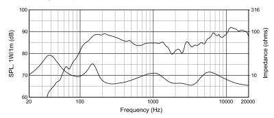
On axis in half-space (2pi, flush mounted in ceiling); Thru (8 W), with Input Impedance
